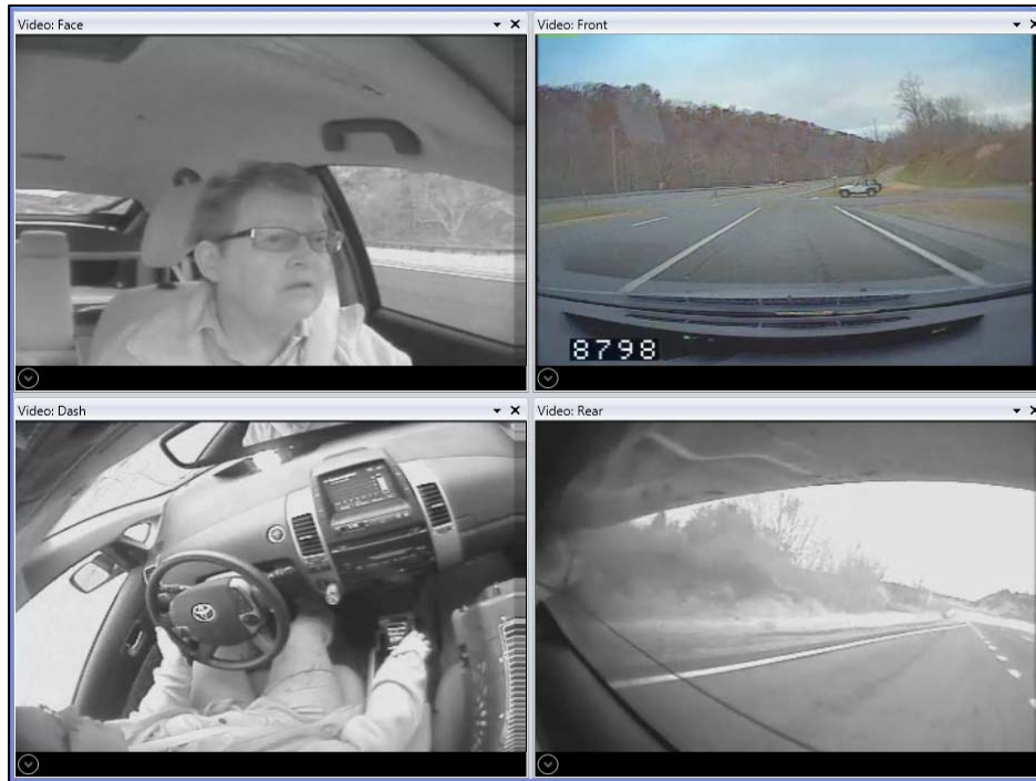
Figure 1. Multiplexed image of the four camera views. Top left: view of the driver’s face. Top right: view of the forward roadway. Bottom left: over-the-shoulder view of the driver. Bottom right: view of the rearward roadway. (Note: Driver shown is a VTTI researcher.)
